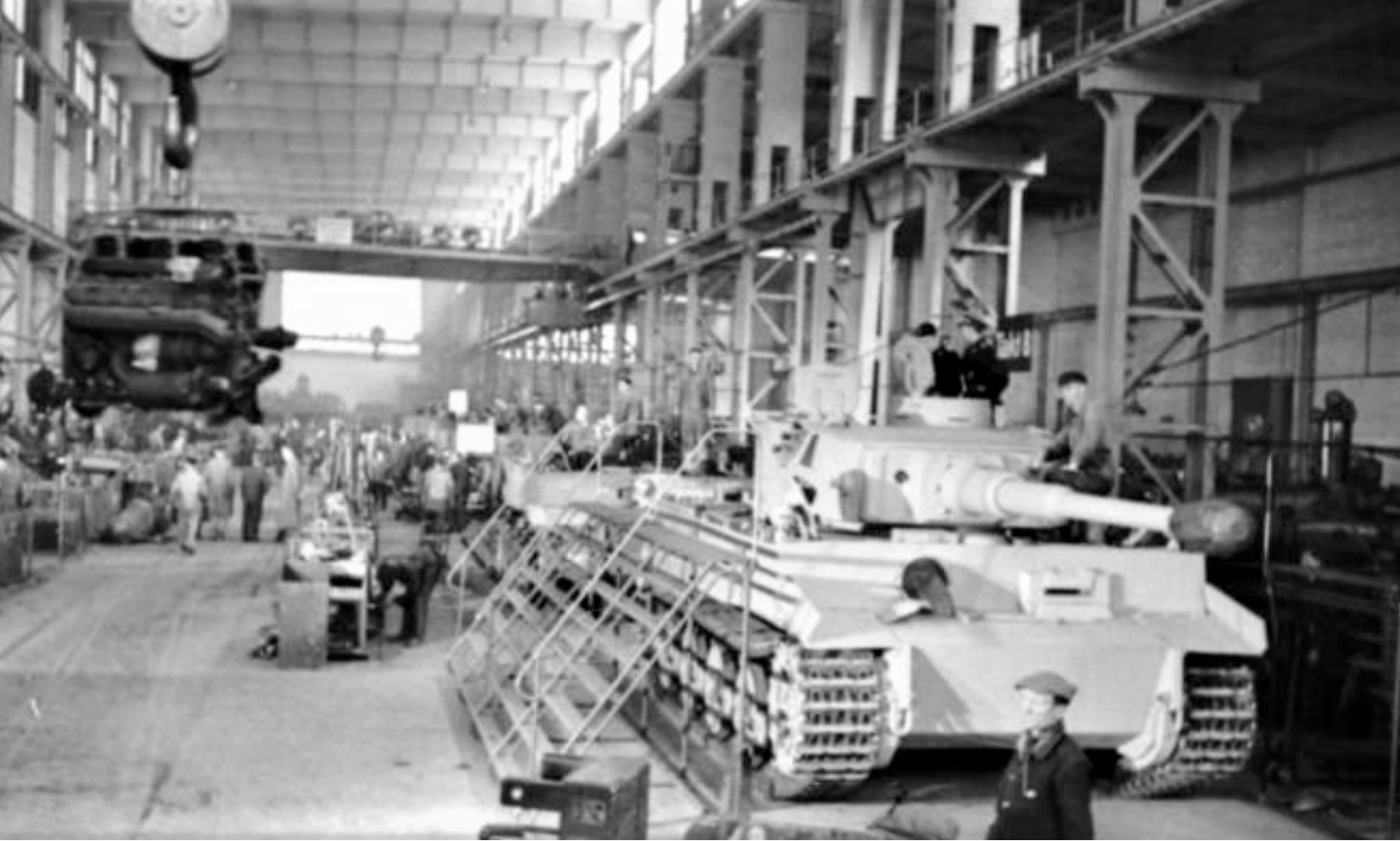
Krupp production of Panzer Tiger I tanks powered by 700 hp at 3,000 rpm, turret armor of 4 inches – German Federal Archives, Wikimedia
