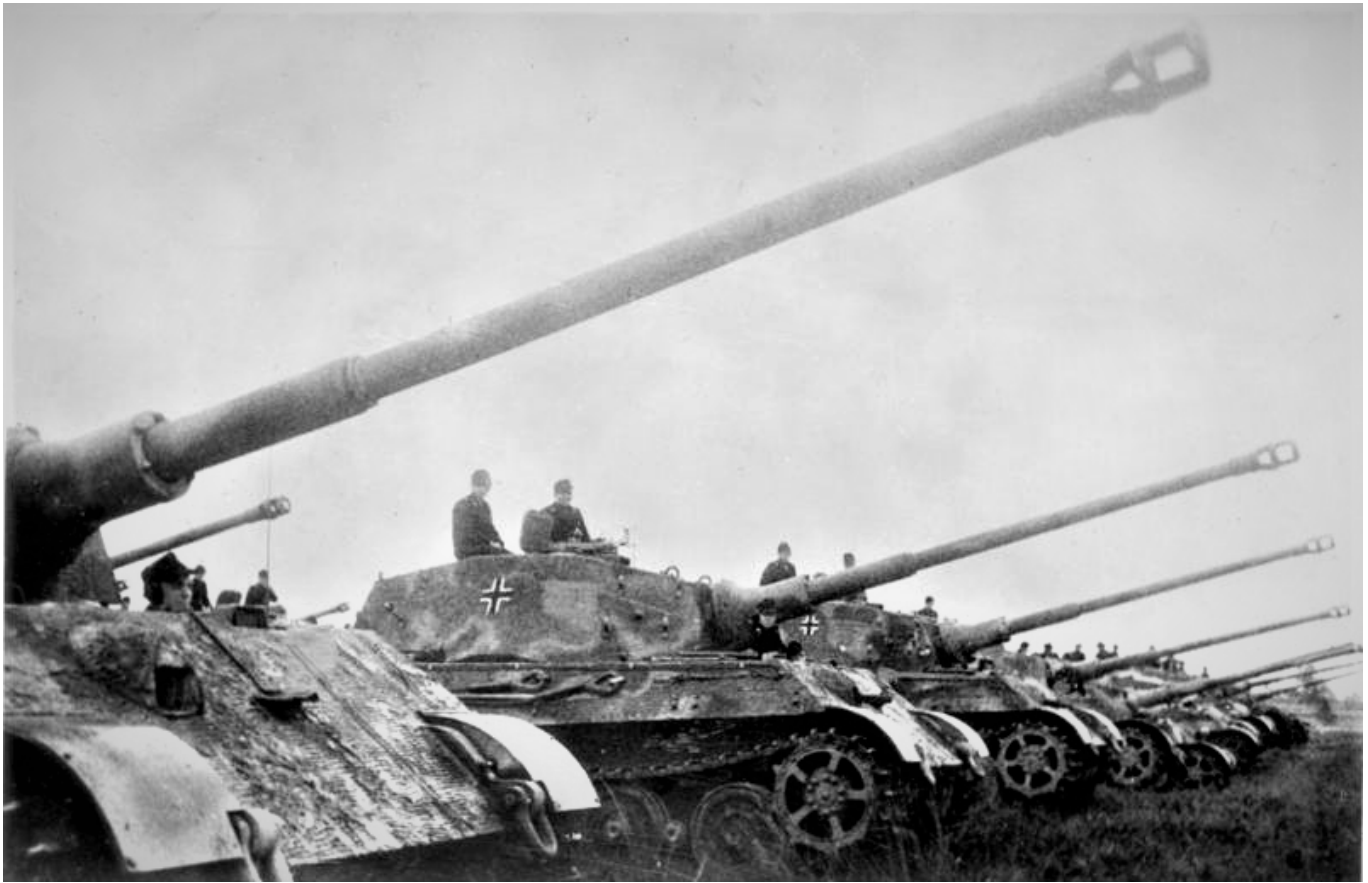
Panzer VI, (Tiger II, Königstiger) weighed 70 tonnes, protected by 4 to 7 inches of armor, armed with the long barrel 8.8 cm KwK 43 L/71 anti-tank cannon – Author, Haman, German Federal Archives, Wikimedia
