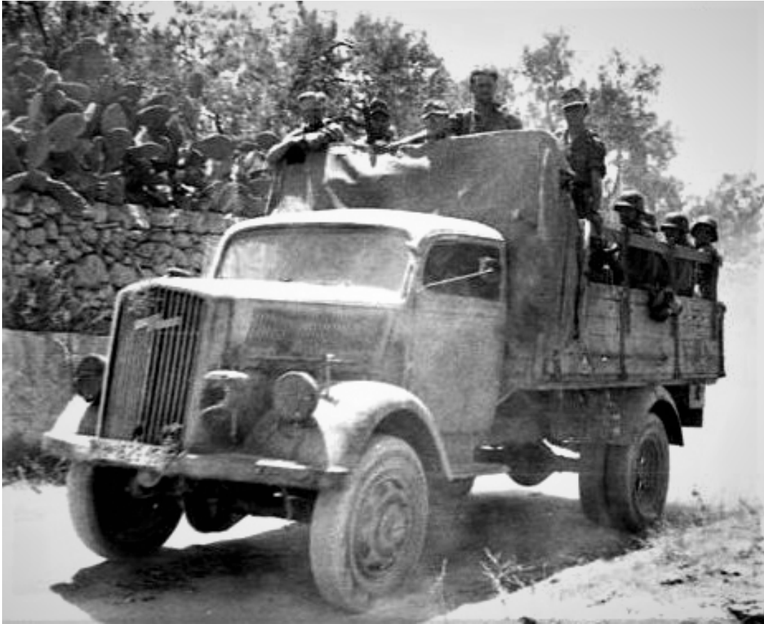
Opel Blitz LKW Wehrmacht truck, Italy, 1944 – Source, Foto Funke cropped from German Federal Archives, Wikimedia. At the beginning of the war, General Motors German subsidiary Opel AG was Germany's largest truck producer. Albert Speer ordered the construction of the Opelwerk Brandenburg factory where until 1944, more than 130,000 Blitz trucks were manufactured. The modern 1937 overhead valve engine was so like Chevrolet engines that disabled three-ton Blitzes abandoned by the retreating Wehrmacht were quickly restored to operation by the Allies using Chevy-GMC parts.
